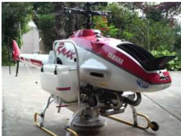
Pictured to the left is the 9-foot Yamaha Rmax. This drone is specifically designed for farmers to use even though it can be used for anything you want. I just want one of these because it looks cool! This is a fully autonomous helicopter that can carry a 62-pound payload and spray 2 acres
