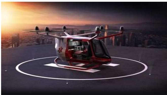
One major step that drones have taken is that a company from Hopkinton, Massachusetts called Alaka'I Technologies has developed a drone prototype that utilizes hydrogen fuel cells which allow the use of electric motors but can be used for a very long
